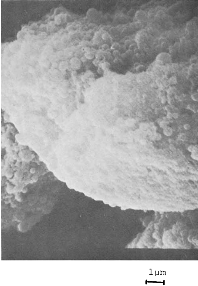
Fig. 8. SEM of fraction 4F: 7,500 \times showing a broken particle.
